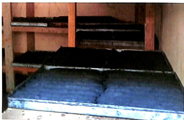
Drying briquettes under shade
